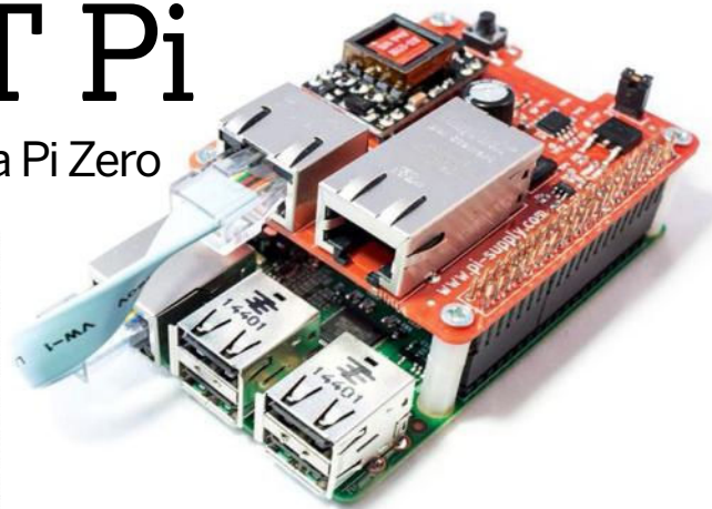
▲ The PoE Switch Hat powers your Pi using an Ethernet cable – but you'll need a suitable PoE injector or switch.
